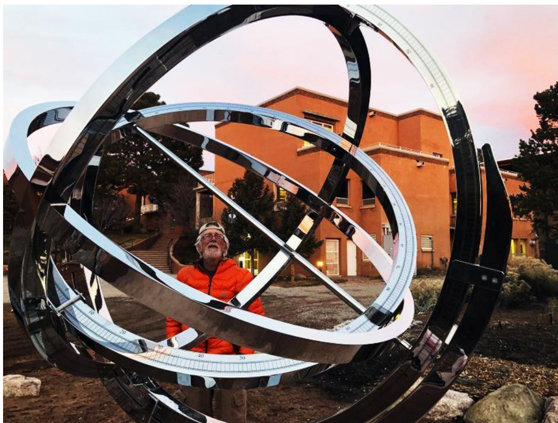
Bill Donahue demonstrates the new functioning replica of Tycho Brahe's Second Equatorial Armillary at St. John's College. The three scales use Brahe's diagonal dot divisions, permitting readings to better than one arc minute. The original was constructed in 1584. Bill reports "We are just beginning to learn how to use this amazing and unique instrument!"
