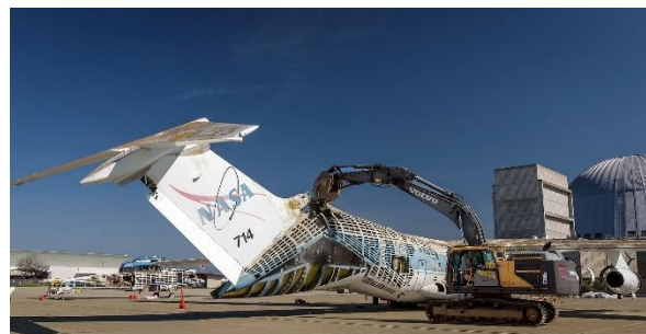
A Volvo Crawler Excavator severs the airframe, separating the tail section from the fuselage, of the modified C-141 Kuiper Airborne Observatory, (KAO) (NASA-714), at Moffett Field, California, on 20 March 2025. (Image credit: NASA Ames, D. Richey, via Wikimedia Commons)
