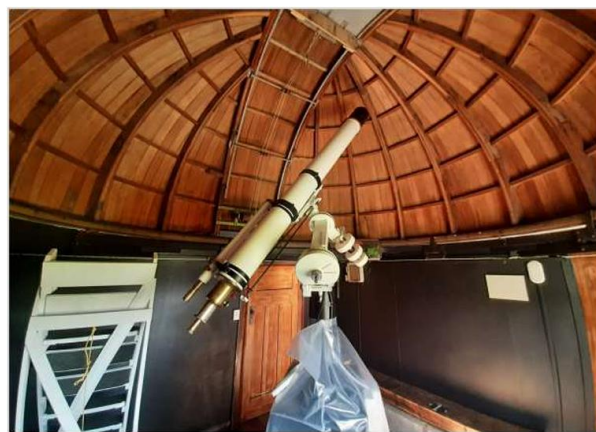
Figure 5: An early 2025 photograph of the refurbished 6-inch ‘Alvan Clark refractor’ back in its original wooden dome at the New Plymouth Observatory. Note that the German equatorial mounting shown here is not original, but in 1921 replaced the makeshift mounting that Gale had provided with the telescope. The current whereabouts of the original Alvan Clark mounting (and perhaps even the tube assembly) is unknown ( Photo courtesy: New Plymouth Astronomical Society ).
